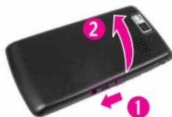
3. Place a fingertip in the cutout to lift the edge of the battery, then remove it.
